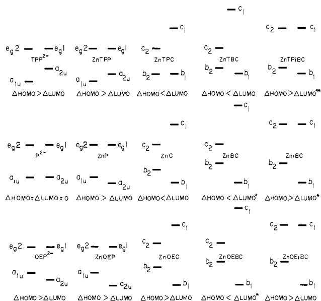
Figure 3. Orbital energy level diagrams added for zinc porphyrins, chlorins, bacteriochlorins, and isobacteriochlorins with use of the protocol developed in the text. The single asterisk denotes predictions not yet confirmed by experiment. The double asterisk indicates a prediction that is inconsistent with experimental results. The source of the inconsistency is discussed in the text.
